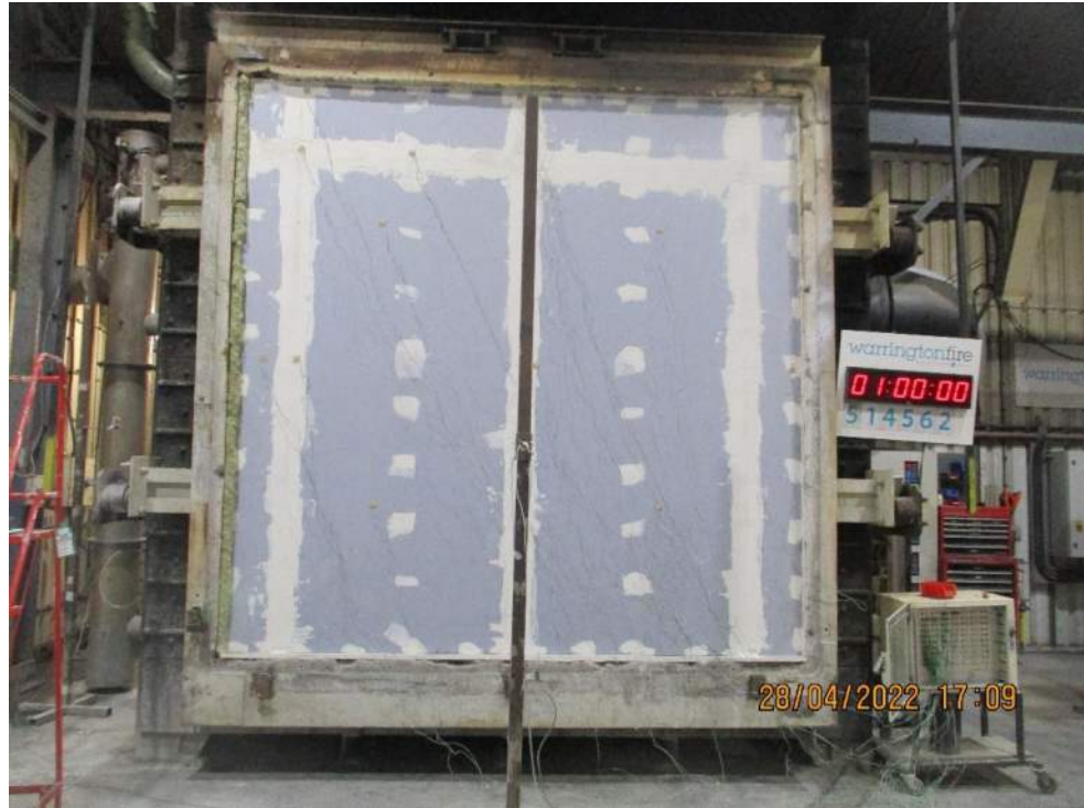
The unexposed face after a test duration of 60 minutes
