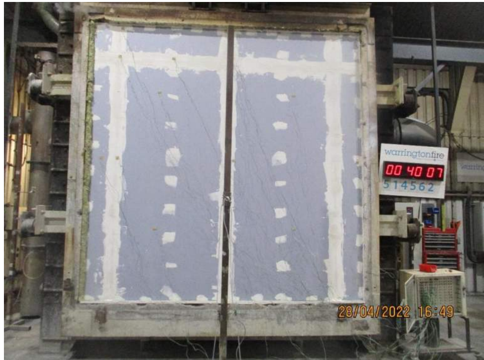
The unexposed face after a test duration of 40 minutes
