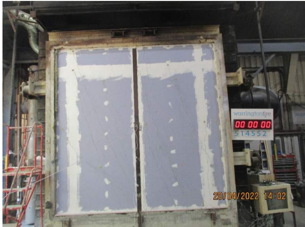
The unexposed face prior to testing
