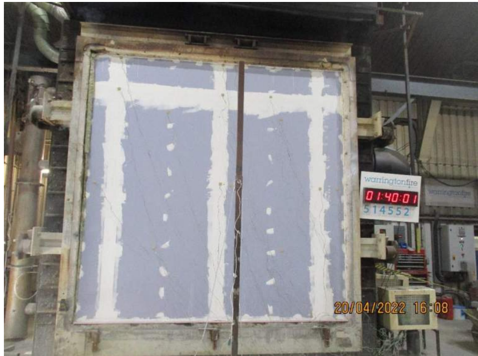
The unexposed face after a test duration of 100 minutes
