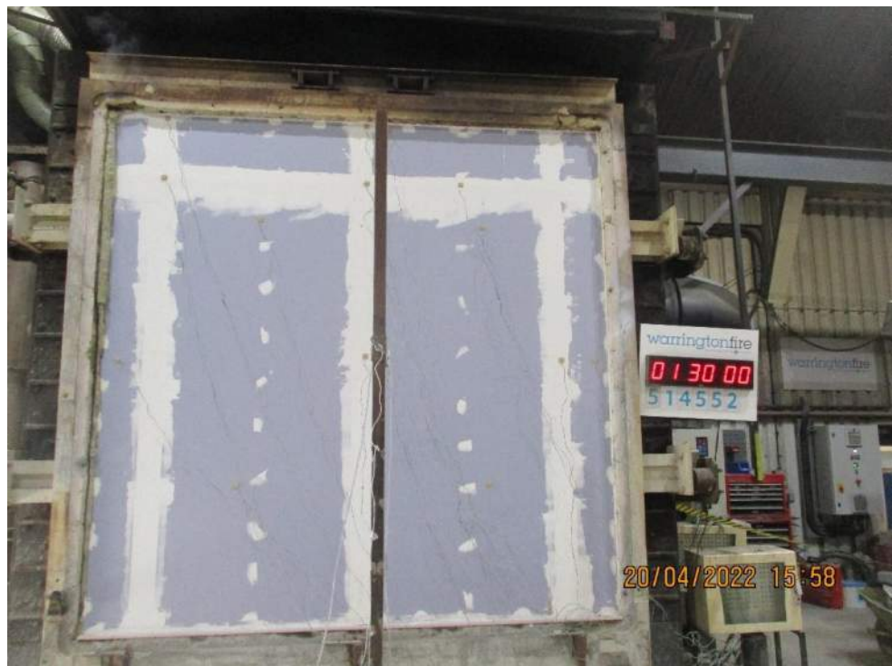
The unexposed face after a test duration of 90 minutes
