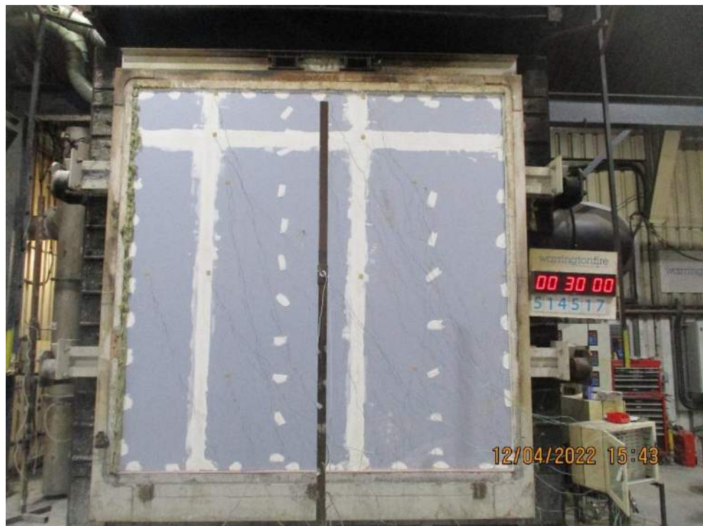
The unexposed face after a test duration of 30 minutes
