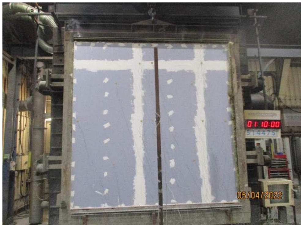
The unexposed face after a test duration of 70 minutes
