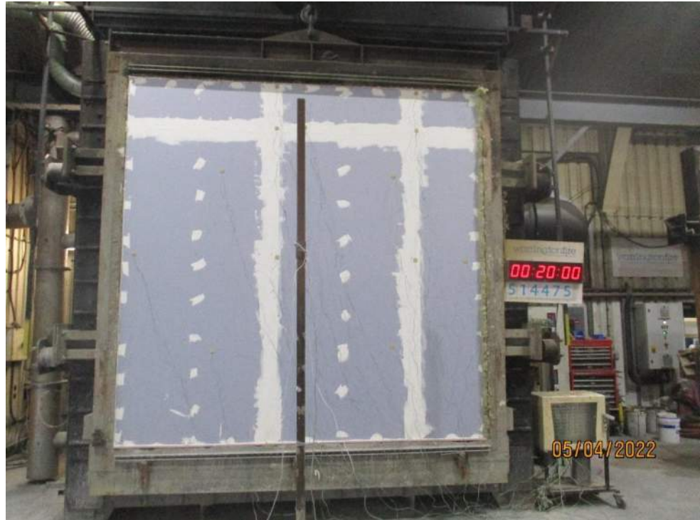
The unexposed face after a test duration of 20 minutes
