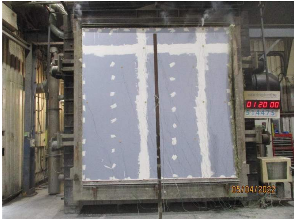
The unexposed face after a test duration of 80 minutes
