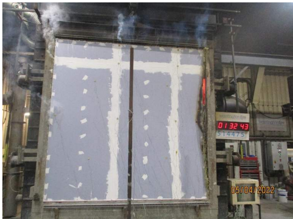
The unexposed face after a test duration of 92 minutes
