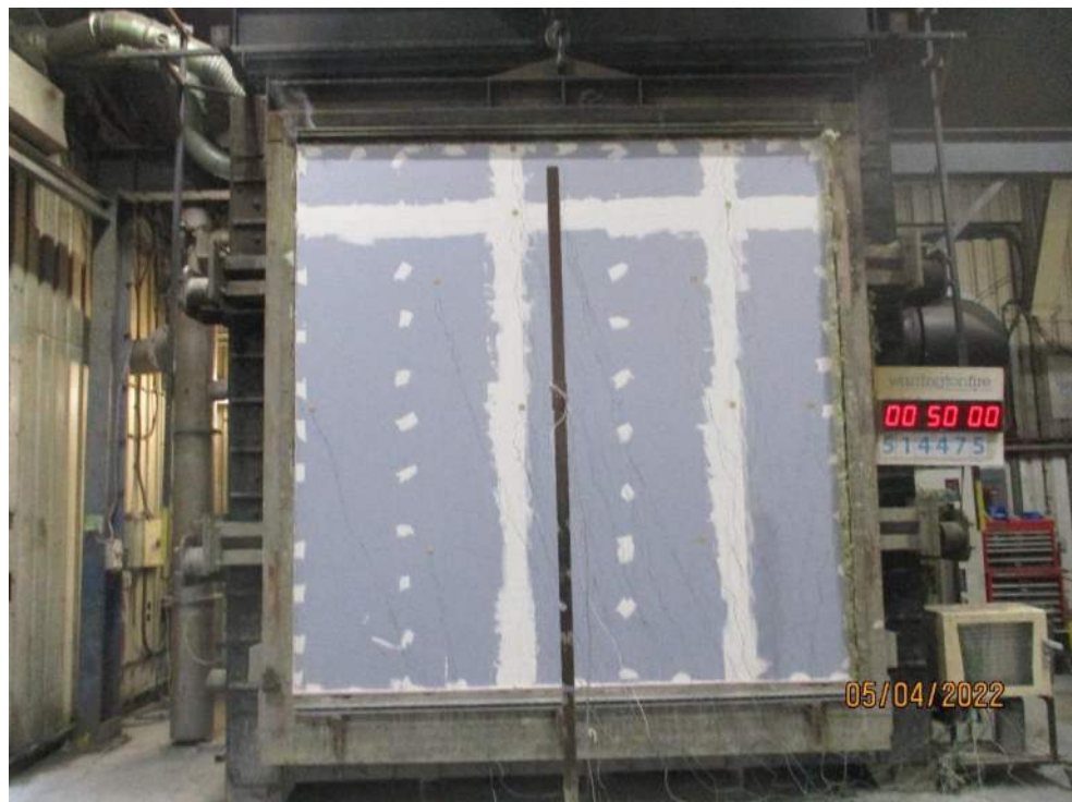
The unexposed face after a test duration of 50 minutes
