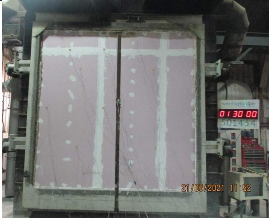
The unexposed face after a test duration of 90 minutes
