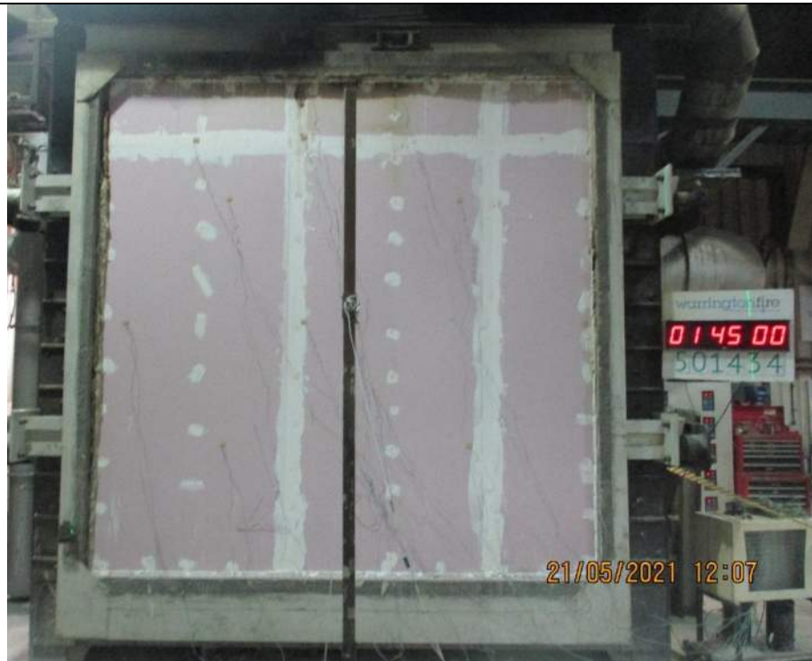
The unexposed face after a test duration of 105 minutes
