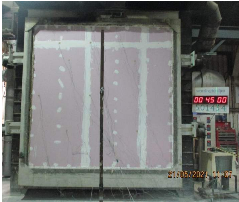
The unexposed face after a test duration of 45 minutes
