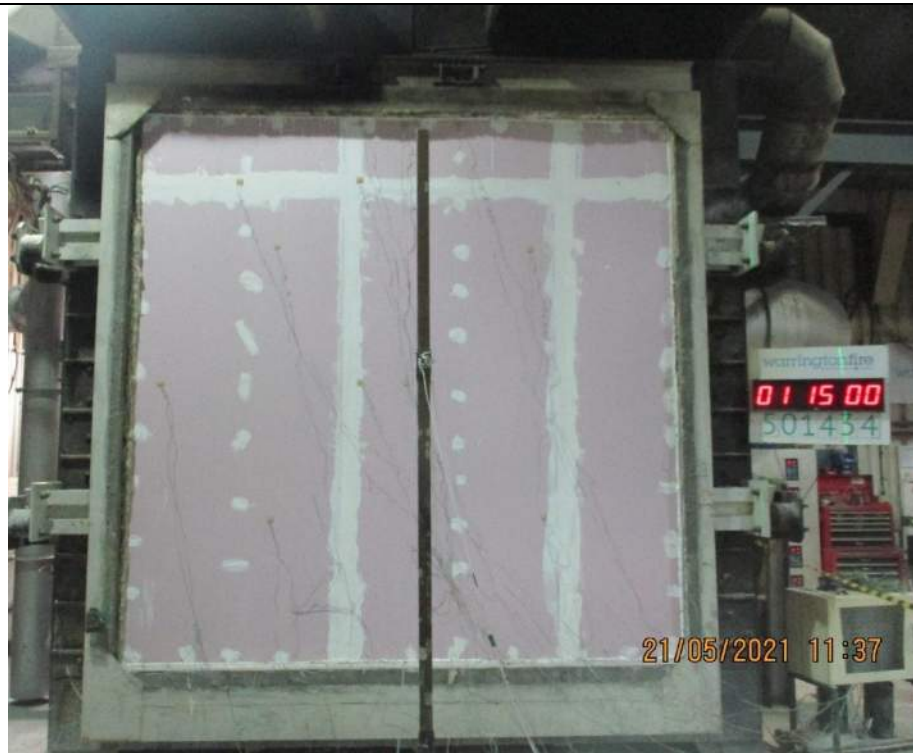
The unexposed face after a test duration of 75 minutes
