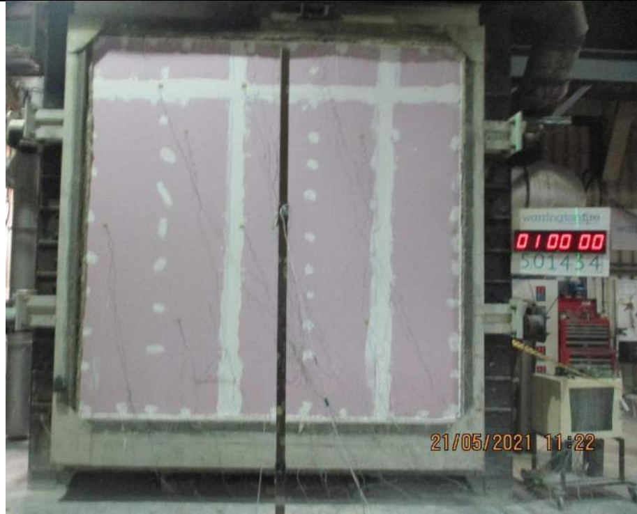
The unexposed face after a test duration of 60 minutes
