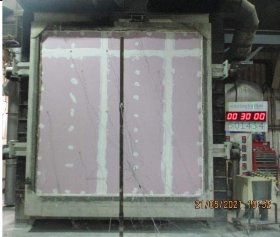
The unexposed face after a test duration of 30 minutes
