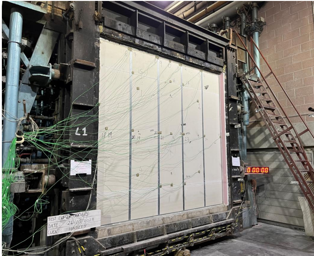
Photo 7 - Unexposed side of the specimen at the beginning of the test
