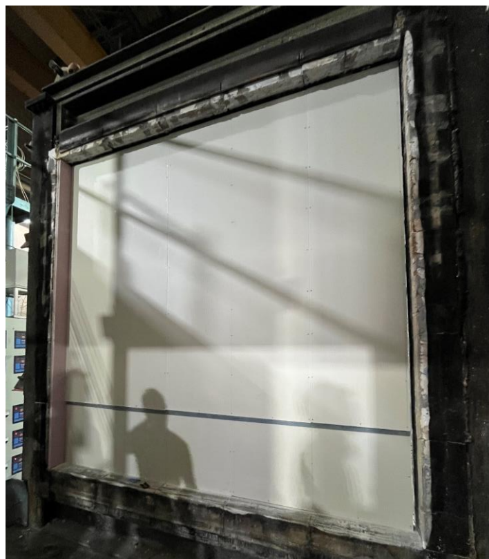
Photo 4 – Second layer of boarding on the exposed side
