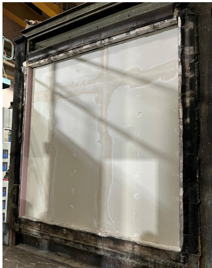
Photo 6 - Exposed side of the specimen before the test
