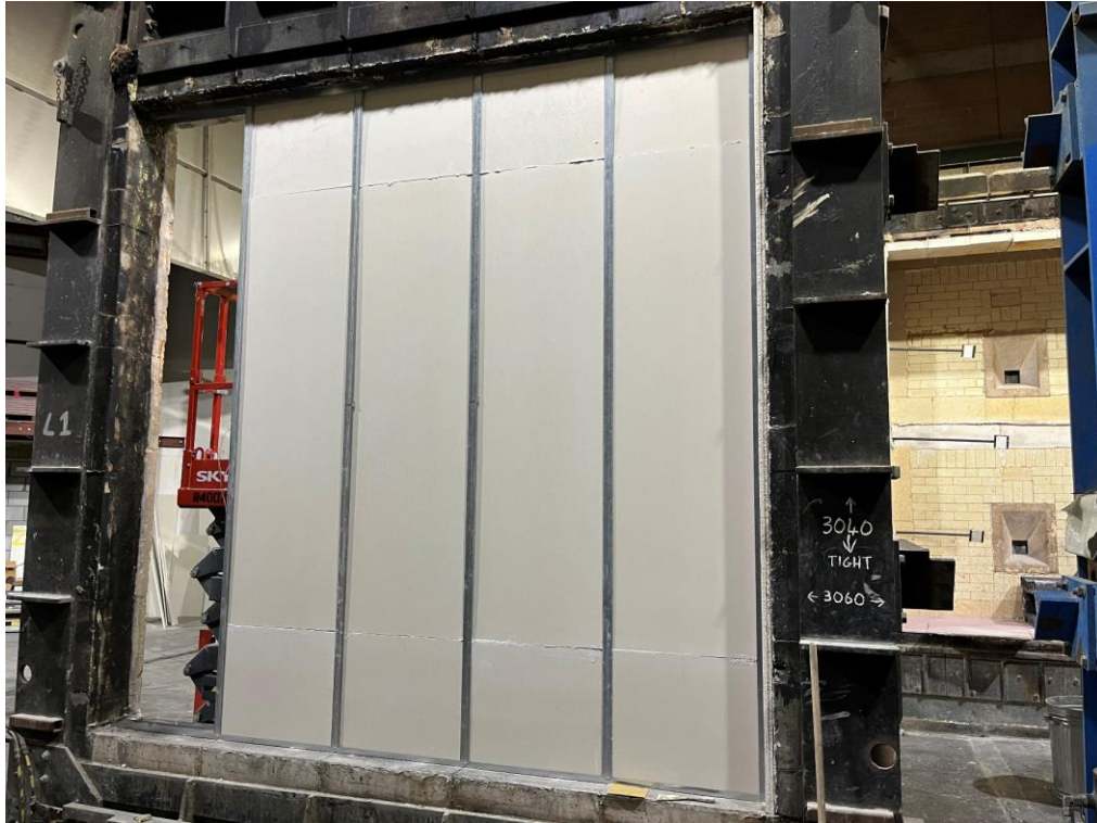
Photo 1 - Specimen During construction – Unexposed side
