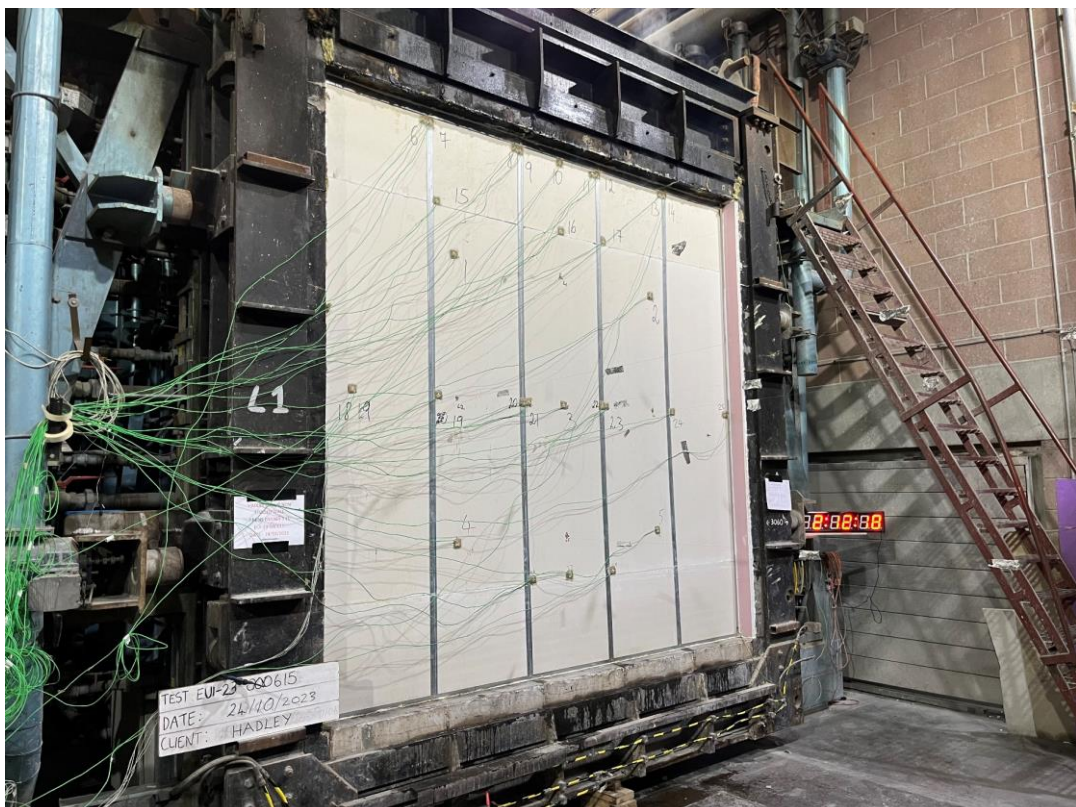
Photo 12 - Unexposed side of the specimen - Min 132 – At the end of the test
