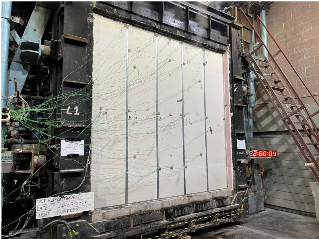
Photo 11 - Unexposed side of the specimen - Min 120
