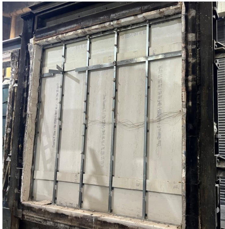
Photo 14 - Exposed side of the specimen during dismantling
