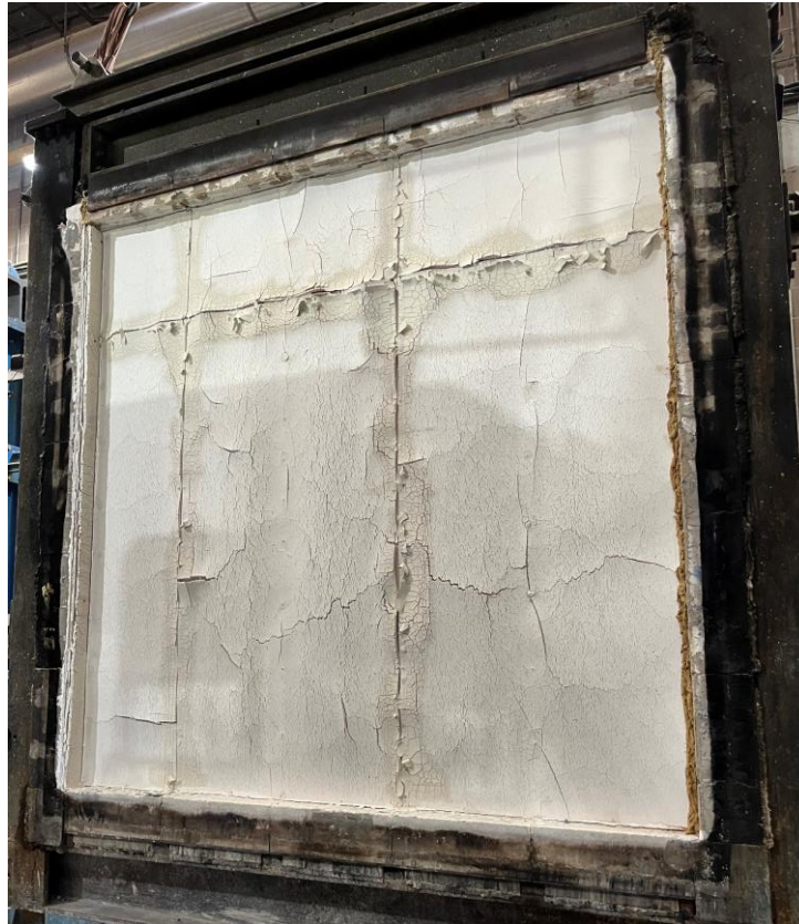
Photo 13 - Exposed side of the specimen after the test
