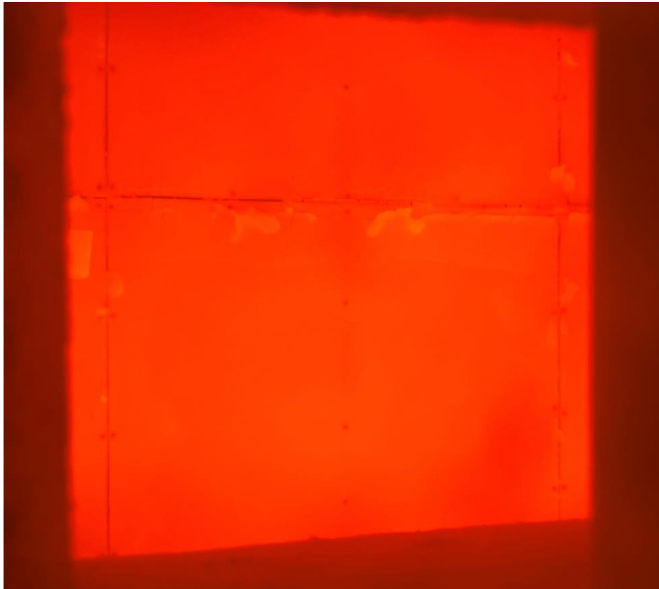
Photo 10 - Exposed side of the specimen - Min 91
