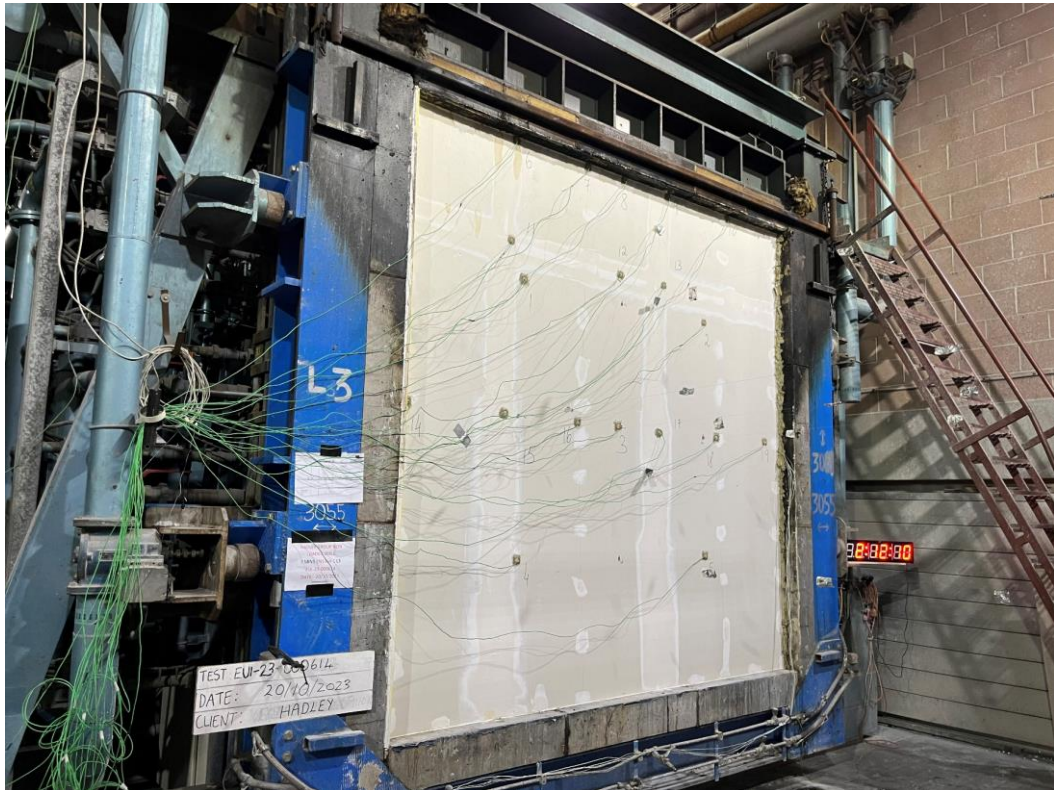
Photo 13 - Unexposed side of the specimen - Min 132 – At the end of the test
