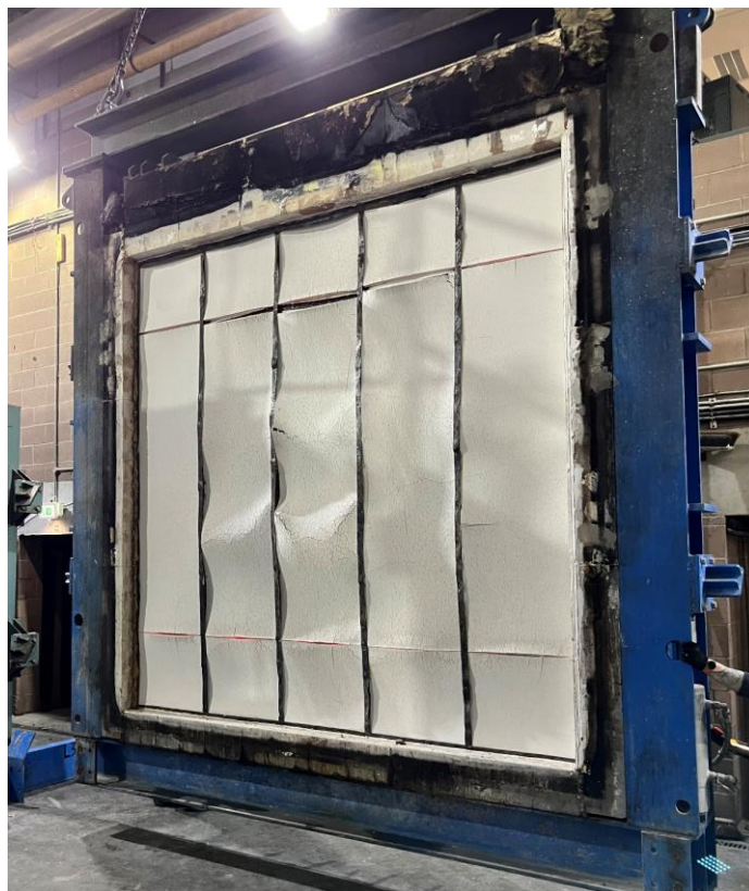
Photo 14 - Exposed side of the specimen after the test
