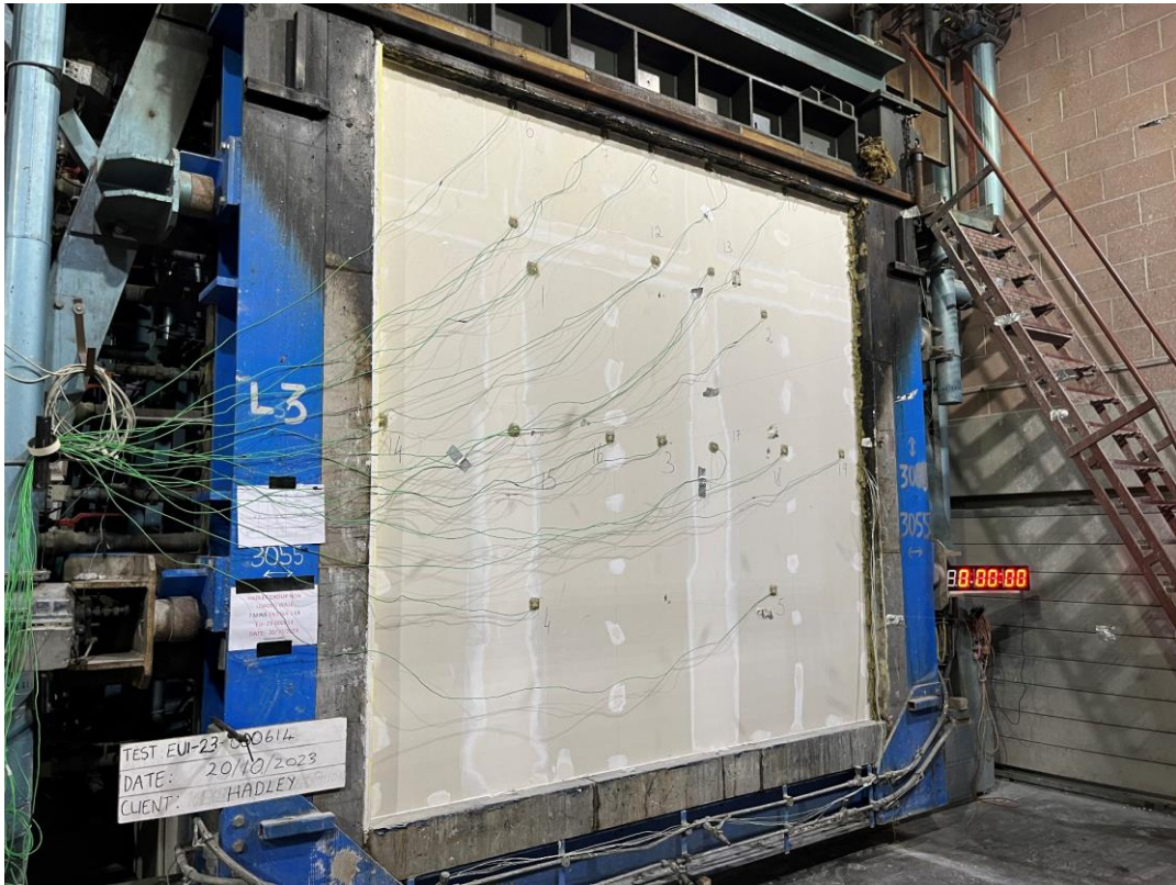
Photo 7 - Unexposed side of the specimen at the beginning of the test
